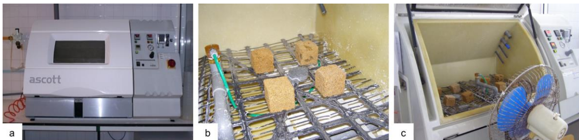
Figure 3. Marine aerosol accelerated ageing test. a) Marine aerosol ageing chamber; b) Drying process without ventilation (6h); c) Drying process with ventilation (6h)
