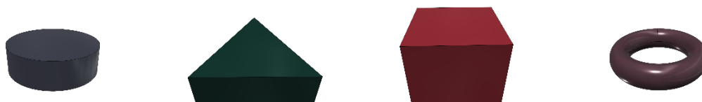
Figure 1. 3D representation of selected geometries of 3DP S-SMEDDS formulations (from left to right - cylindrical, prism, cube and torus). The objects were drawn using AutoDesk 123D Design software (Autodesk Inc. USA) for printing as described.
