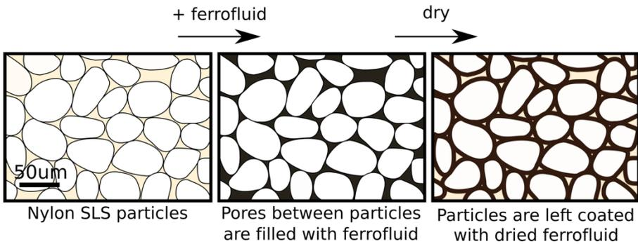
Figure 2: Schematic cross-section of the post-processing method, where SLS prints were dipped in ferrofluid and then dried. The process deposits magnetic nanoparticles in the form of dried ferrofluid throughout the porous material.
