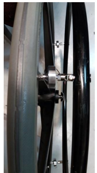
Fig. 5. Three slaves connecting pushrim with drivewheel.
