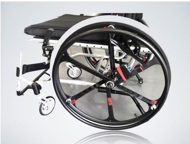
Fig. 1. Sensewheel slave load cells mounted at 120deg intervals around the wheel, wired to the hub master, fitted to a VanOs Excel 2 wheelchair.
