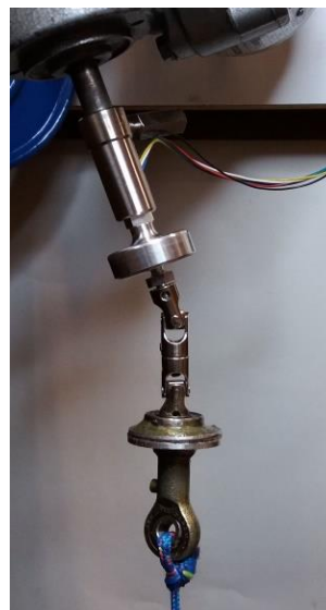
Fig. 4. Slave angled and rotated about axis to calibrate with known axial and shear forces.
