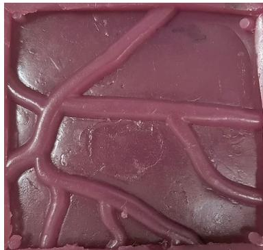
Figure 3. Top down photograph of the tissue mimicking gel wax placenta phantom.
