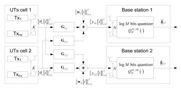
Fig. 4. Massive MIMO channel estimation with  $n_c = 2$  cells.
