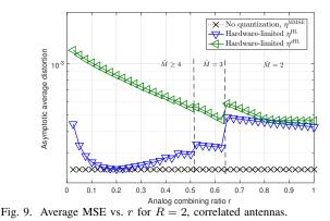
This follows since properly combining correlated samples from different time indexes results in an error which is negligible compared to that induced by the uniform quantizers, hence, hardware-limited quantizers with general analog combining operate best when the analog combining decreases the number of quantized samples to be not larger than the number of channel coefficients, i.e.,  $r \leq \frac{K}{L}$ , allowing the quantization to be carried out with improved resolution.
