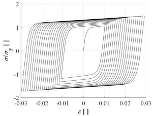
Figure 4: Cyclic response of the steelBRB material under sinusoidal history with increasing amplitude.
