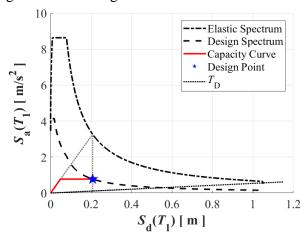
Figure 3: Performance point of the equivalent SDOF.
