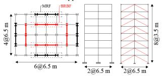
Figure 1: Case-study building: plan view (left) and elevation view of the MRF and BRBF (right).
