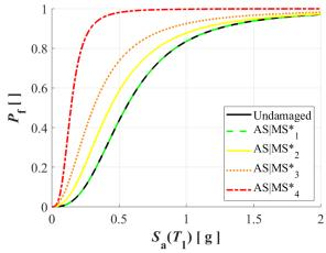
Figure 10:  $\mu_c$ -based AS fragility curves, conditioned to the level of damage induced by  $MS^*_{i}$ .
