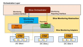
Figure 2: SMA Implementation using Lattice
