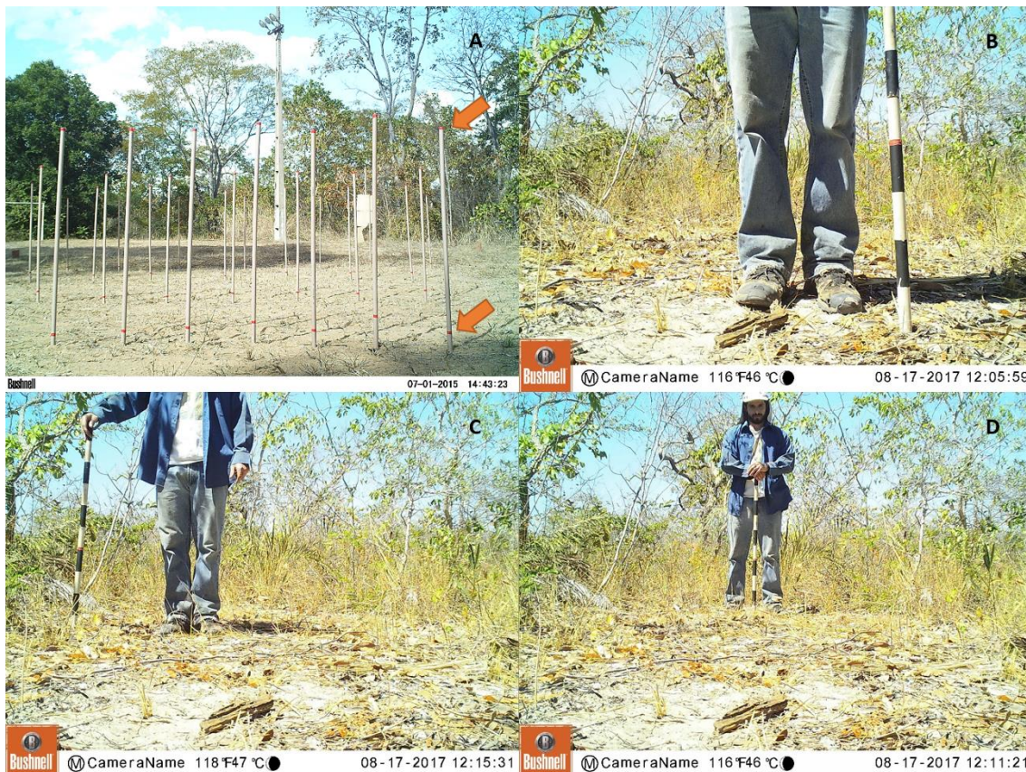
Figure 5.3: Calibration procedure that enables extracting distance and angle from camera trap images of animals. A) Camera calibration with 28 1-m poles equally distributed in four rows located at 3, 5, 7 and 9 m from the camera trap. Length of the segment between red bands (indicated by arrows) is 90 cm. B-D) Examples of site calibration pictures using a 1-m pole marked with 10-cm black and white bands. Approximately 15 pictures at distinct positions covering the camera's field of view were taken at each sampling site.
