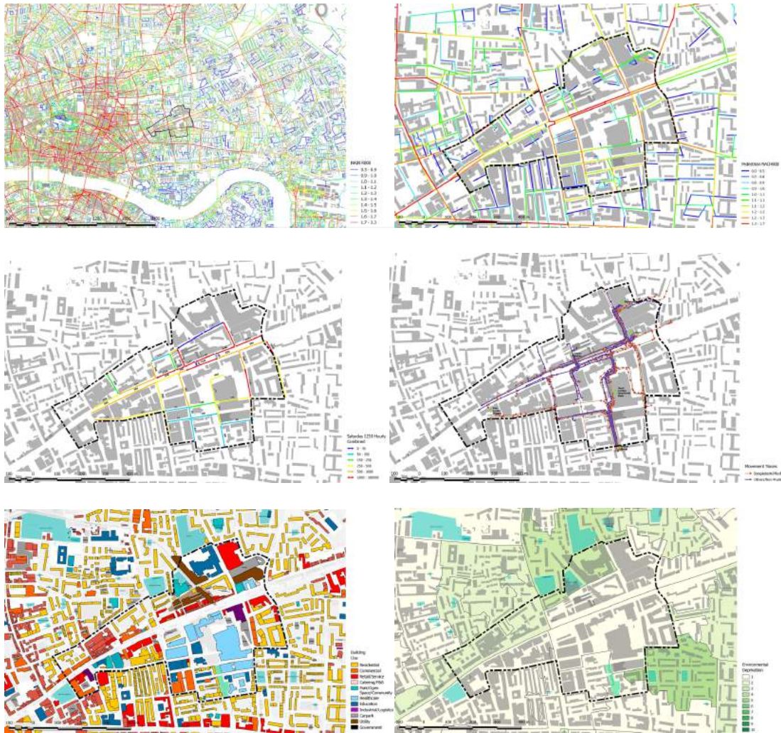
Figure 7: Segment angular analysis (top left), high resolution segment angular analysis (top right), pedestrian movement flow analysis (middle left), pedestrian trace analysis (middle right), land use analysis (bottom left), access to public amenities analysis (bottom right).
