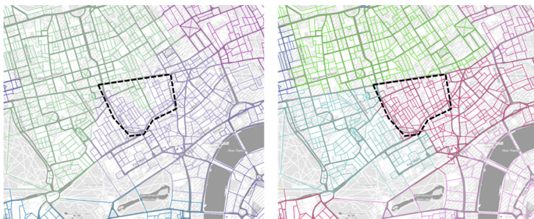
Figure 10. Comparing Connectivity-weighted local area and Betweenness-weighted local area for Soho in London.
