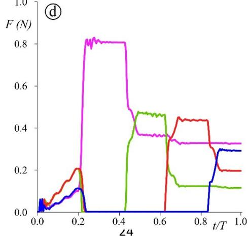
451 **Figure 7.** Force applied by neochords during the implant in **a)** *AT strategy*, **b)** *1by1a (central to lateral*
