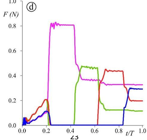
443 **Figure 7.** Force applied by neochords during the implant in **a)** *AT strategy*, **b)** *1by1a (central to lateral*
