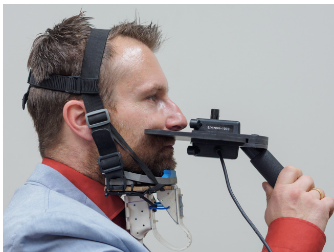
FIG. 3. (Color online) An example of the experimental setup used in the study, including a hand-held Glottal Enterprises nasalance device and an ultrasound probe holder headset (Derrick et al. , 2015).
