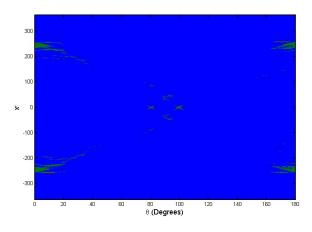
Fig. 8. The result of applying Radon transform on frequency wavenumber domain (positive and negative frequecy are considered).
