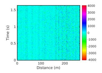
Fig. 1. Sample of raw acoustic data in distance (horizantal axis) and time (vertical axis).
