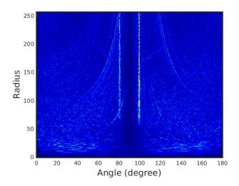
Fig. 6. Polar representation of acoustic data in frequecy wavenumber domain.
