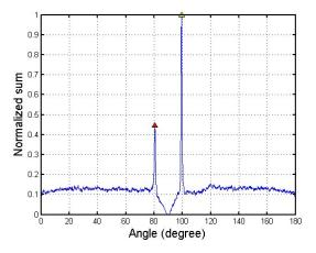
Fig. 7. Summation along the radius. Two peaks shows the location of the two lines.
