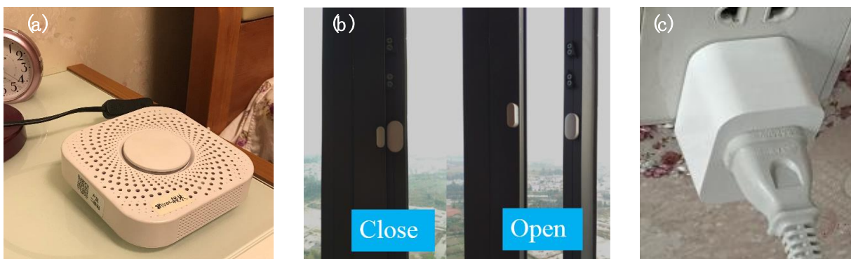
13 14 Figure 2: Monitoring instruments: (a) An environmental monitoring kit for indoor air 15 temperature, humidity and CO 2 concentration; (b) Magnetic contactors for monitoring 16 window states; (c) A socket for monitoring air-conditioner power consumption 17
