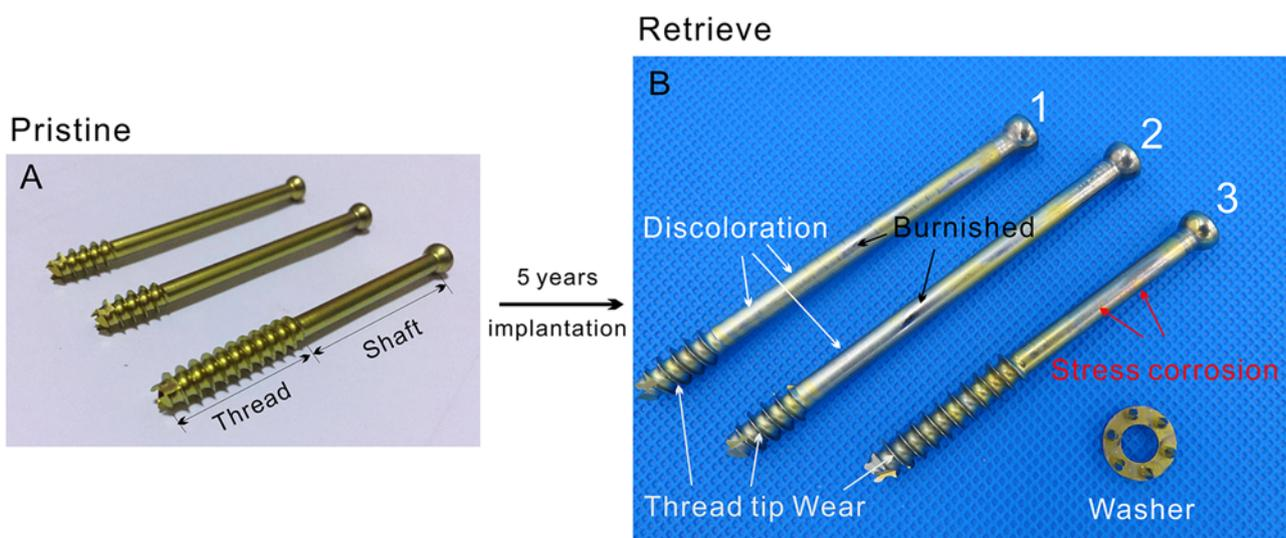
**Fig. 2** Comparison optical image of pristine screws and degradation of screws
