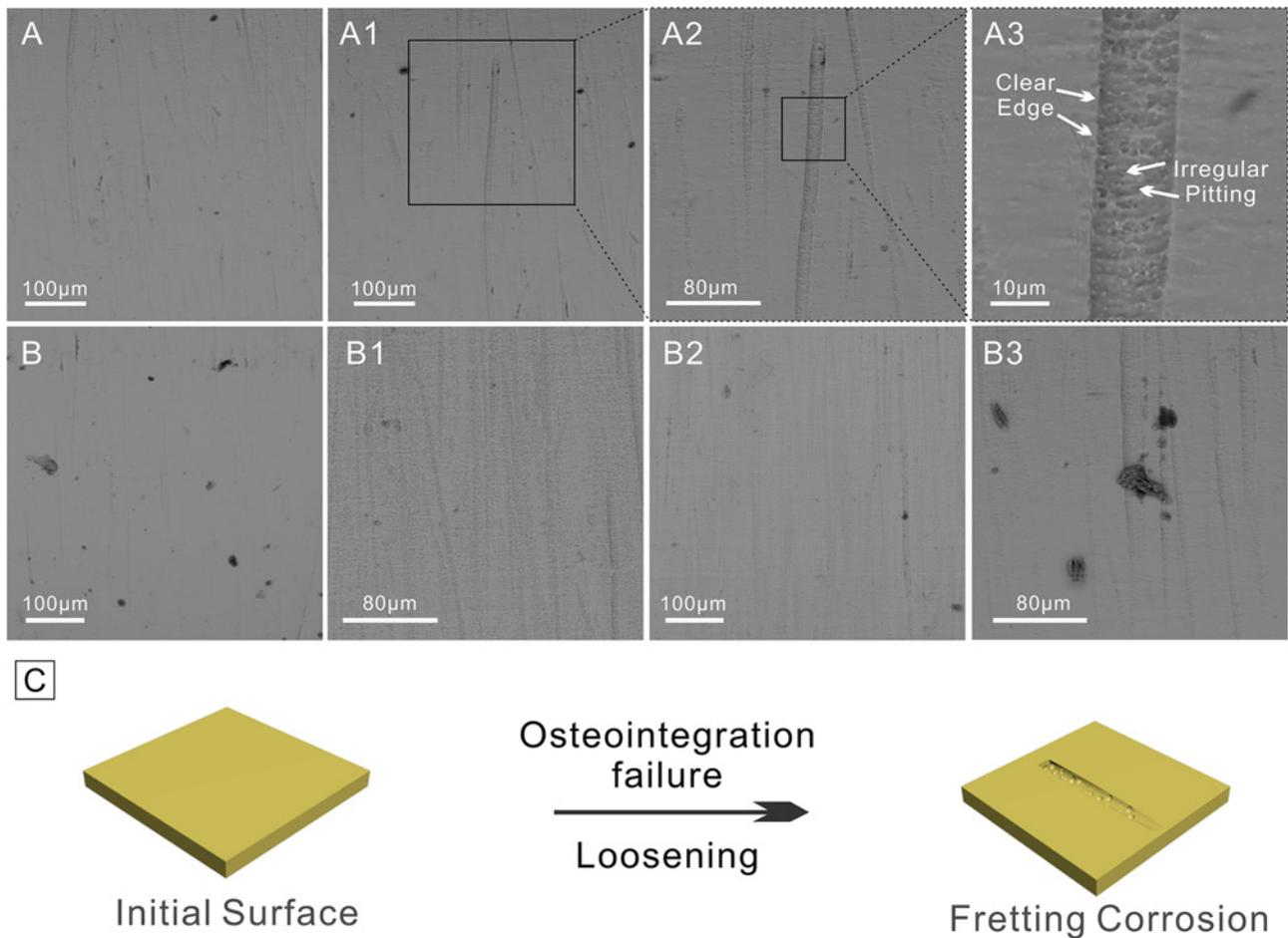
**Fig. 3** SEM images of shaft areas on screw 1
