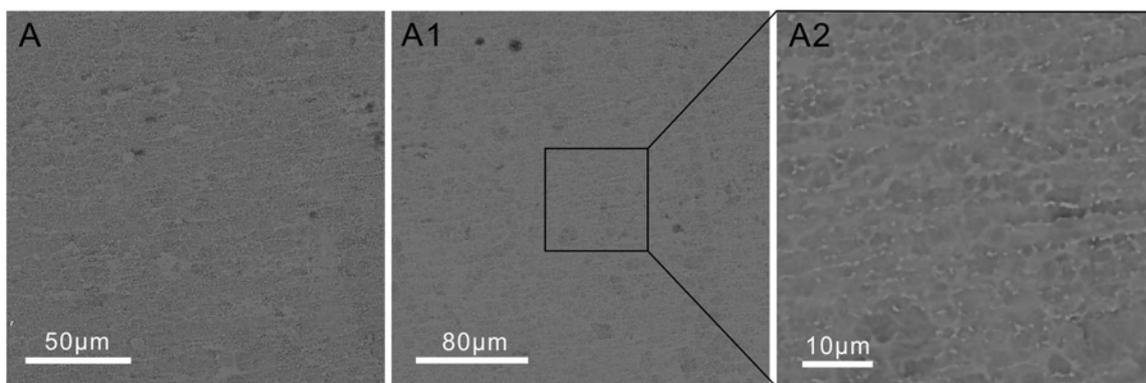
**Fig. 4** Fretting corrosion morphology features on screws 1 and 2 shiny (burnished) areas
