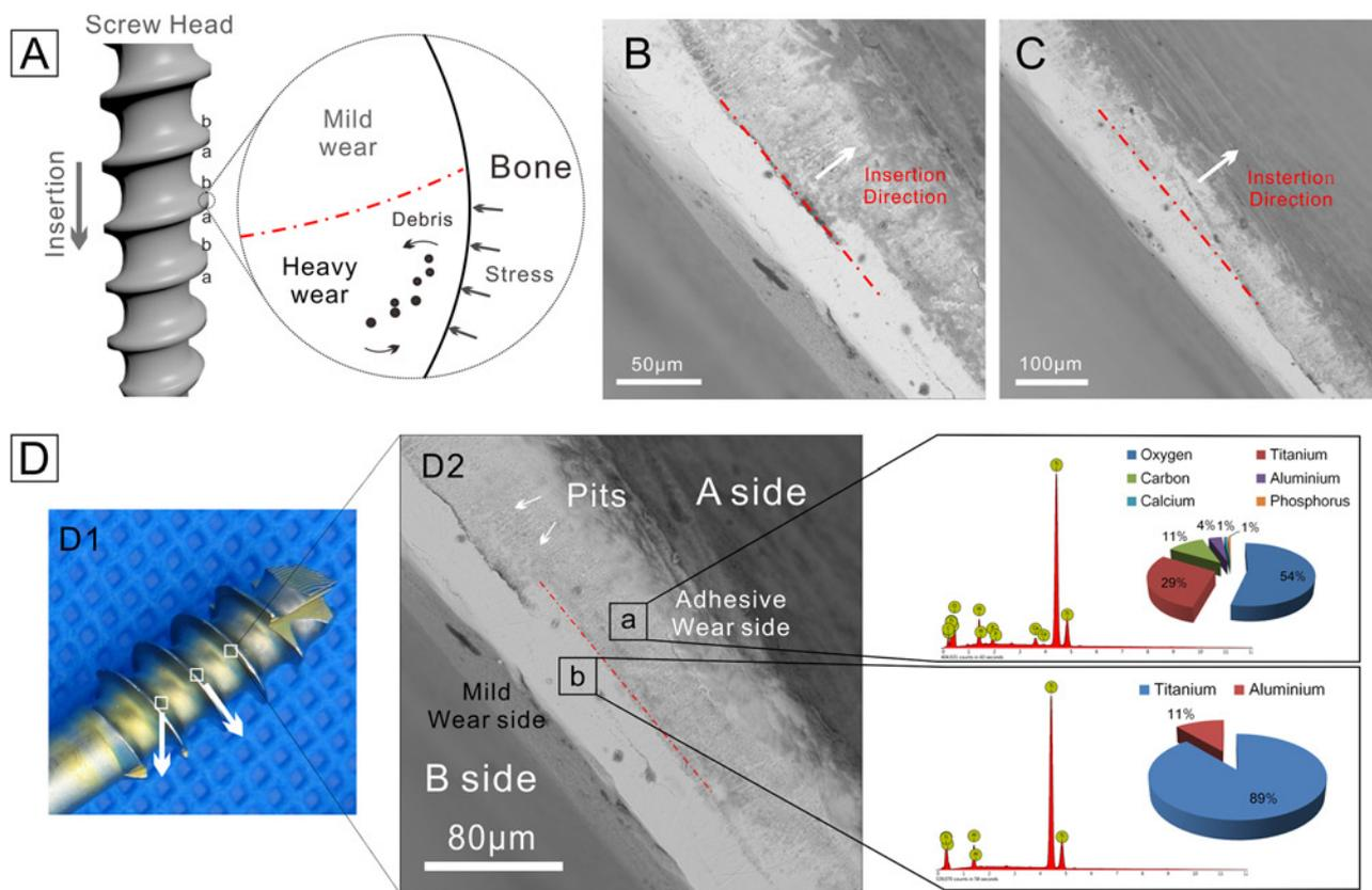
**Fig. 7** Schematic images of insertion wear
