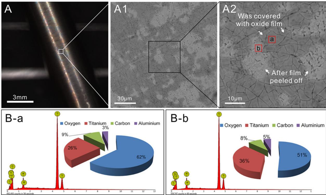
**Fig. 5** Stress corrosion on screw 3
