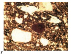
Plate 47 Thin-section photomicrographs of medieval ceramics from the Hedingham pottery industry. A. Coarseware fabric howstor. B. Rounded sand temper, C. Rounded sand temper, parallel elongate voids and high optical activity, D. Clay rich textural feature which may be unmixed base clay, E. Foliated, metamorphic polycrystalline quartz, F. Small rounded orange amorphous weathered inclusion. All images taken in XP, except F–PPL. Image width A = 1.25 cm, B–D = 3.8 mm, E = 2.4 mm, F = 1.0 mm
