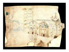
Drawing on vellum might appear antiquated, but in the Middle Ages architectural designs on a membrane were a technological innovation. Its use is a paradox: it constitutes the first materialization of architectural representation, as well as a significant step away from matter.
