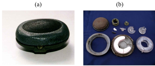
Fig. 8. Neutralized landmine. (a) External view. (b) Disassembled target [11].
