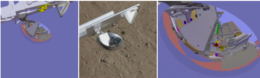
Fig. 5. Images of the RIM, comparing a simulated image produced using AUPS (left) and an image captured by AUPE during a field trial (center) demonstrates the visual fidelity of the images. Right, a closer view of the RIM image, cropped from the original image shown on the left. PanCam is visible at the top of the mirror looking down.
