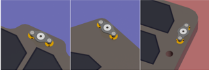
Fig. 7. The three FidMs as seen by HRC in their different locations on the rover deck. The FidMs will be used to geometrically calibrate PanCam once the mast has deployed, ensuring it has unfolded correctly.
