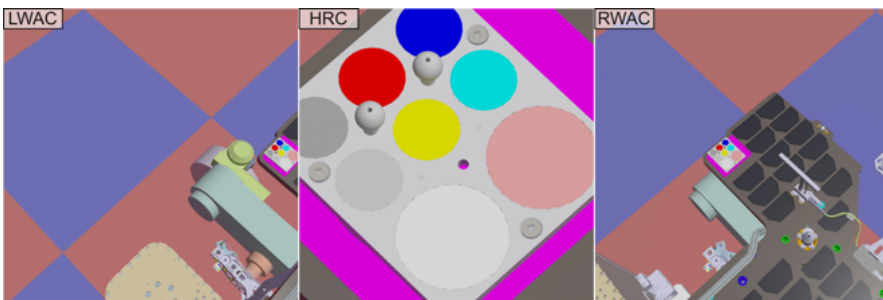
Fig. 4. A set of three images produced by AUPS where HRC has been aimed directly at the centre of the PCT, producing the accompanying Left and Right WAC images. In this configuration, the PCT patches are almost fully visible to HRC, the PCT is centred in the right WAC, but is very close to the edge of the left WAC.
