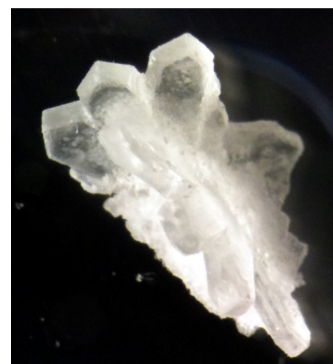
Figure 1. A cluster of platy \text{MgSO}_4 \cdot 3\text{D}_2\text{O} crystals; the field of view is approximately 6 mm wide.
