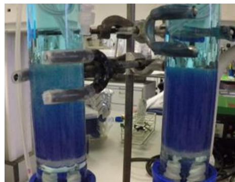
Figure 10 – Fluidisation of alginate beads with different compositions in the sFBB. Left bioreactor contained 50% alginate cell beads and 50% alginate empty beads, while the bioreactor on the right was solely composed of cell beads.
