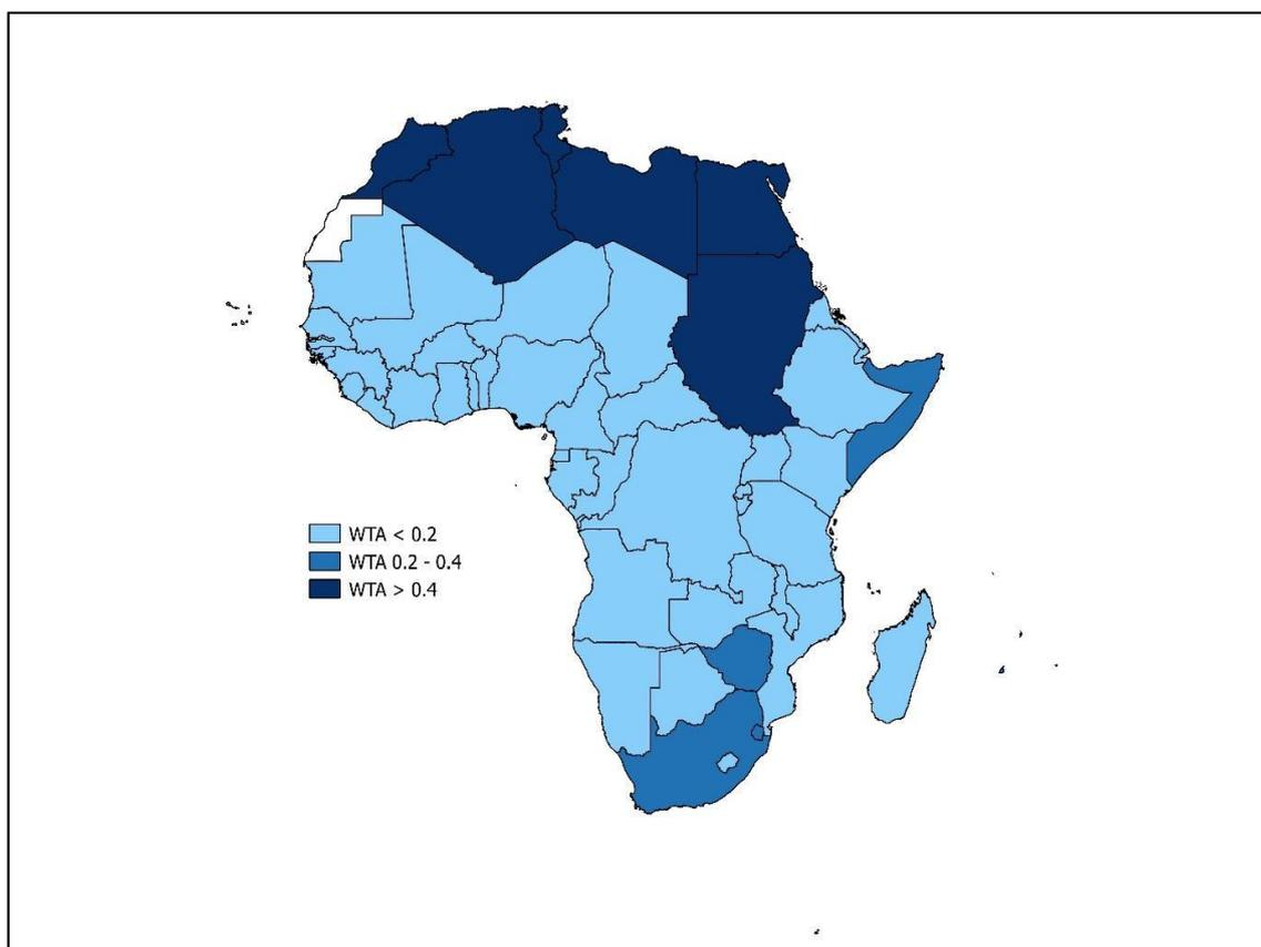
Figure 2.6: Map of national-scale water scarcity as defined by the Withdrawal-To-Availability (WTA) ratio across Africa using data from 2000-2002 (FAO AQUASTAT).
