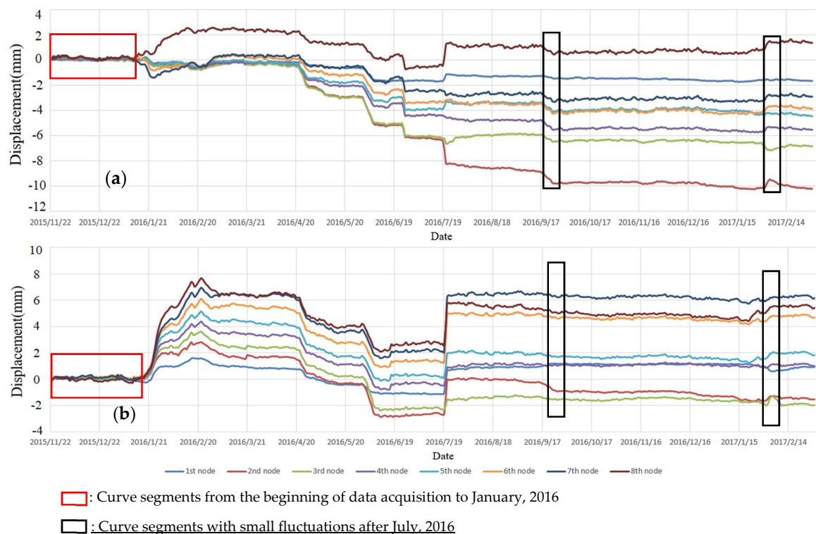
Figure 6. Curves of cumulative horizontal displacement in the X and Y directions of the 4 m-long SAA. (a) Curves of cumulative horizontal displacement in the X direction of the 4 m-long SAA; (b) Curves of cumulative horizontal displacement in the Y direction of the 4 m-long SAA.
