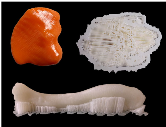
FIG. 5—Photographs of three 3D printed replicas illustrating striations on the surface (upper-left), build raft (upper-right), and support scaffolding (lower). [Color figure can be viewed at wileyonlinelibrary.com ]
