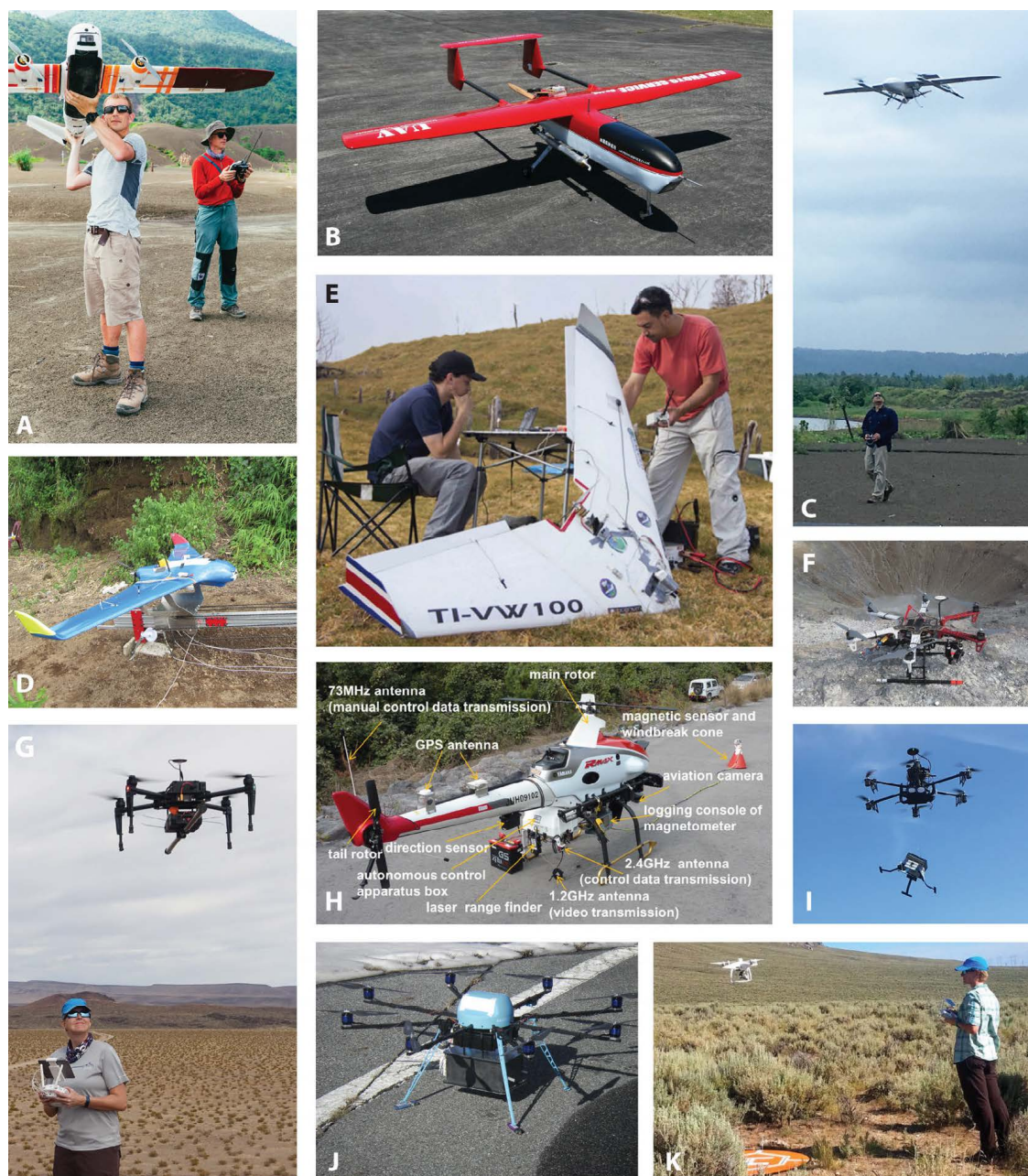
Figure 1: Examples of UAS platforms. [A] A 2.2-m-wingspan fixed-wing Skywalker Titan airframe with custom avionics, used for long-range aerial gas measurements at Manam, Papua New Guinea. [B] A 2.8-m-wingspan aircraft from Air Photo Service Inc., Japan used for imaging lava flow activity on Nishinoshima island [Nakano et al. 2014]. [C] A Foxtech Baby Shark quad vertical takeoff and landing (VTOL) aircraft, used for gas measurements at Tavurvur, Papua New Guinea. [D] A fixed-wing Skywalker X8 with custom avionics, used for ash sampling at Volcán de Fuego, Guatemala [Schellenberg et al. 2019]. [E] VectorWing 100 at Turrialba, which has undertaken autonomous \text{SO}_2 concentration measurements in the plume at maximum altitudes of >3.5 km [Pieri et al. 2013a] [F] DJI F550 hexacopter, with a consumer-grade Sony NEX-5T camera used for photogrammetric campaigns over La Fossa cone, Vulcano (Aeolian Islands, Italy). [G] A DJI Matrice 100 with a Sensys MagDrone R3 aeromagnetic sensor, surveying buried lava flows and cinder cones at Crater Flats, Yucca Mountain, Nevada, USA. [H] The RMAX-G1 used for aero-magnetic measurements and seismometer deployments at Kuchinoerabujima, Japan [Ohminato et al. 2017] [I] Custom-built hexacopter carrying sensor pod ( \text{CO}_2 , P, T, Rh) for remote deployment and retrieval at Rabaul, Papua New Guinea (credit: Jones, J., and Fricke, G.M). [J] \alpha UAV-series octocopter, used at Mt. Ontake for multi-GAS measurements (black box), note also the white adhesive sheet for particle sampling (reproduced from Mori et al. [2016] under the Creative Commons Attribution 4.0 International License). [K] A DJI Phantom 4 RTK used for photogrammetry in the Lost River Range, Idaho, USA.
