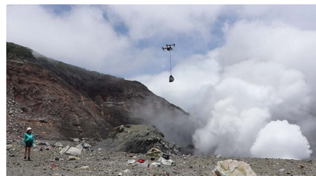
Figure 17: CO 2 sampling from the plume at Poás volcano, Costa Rica (2019). The gas sampling payload (550 g) is suspended 1.5 m below the DJI Inspire 1 as it is flown into the plume. The sample is procured by a remotely operated pump which fills gas bags for isotopic analysis in the laboratory.
