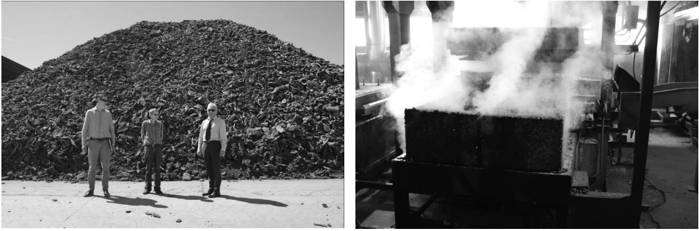
Figure 8. Left: Pile of cork by-product ready for processing, Amorim, Portugal, 2016. Photographer: Oliver Wilton. Right: Two ‘freshly baked’ pure expanded cork blocks emerging from the autoclave, Amorim, Portugal, 2015. Photographer: Matthew Barnett Howland.
