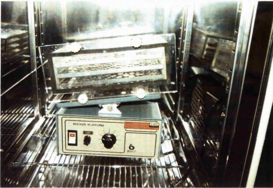
Figure 3. The organ culture chamber sealed and placed on a rocking platform within an incubator.
