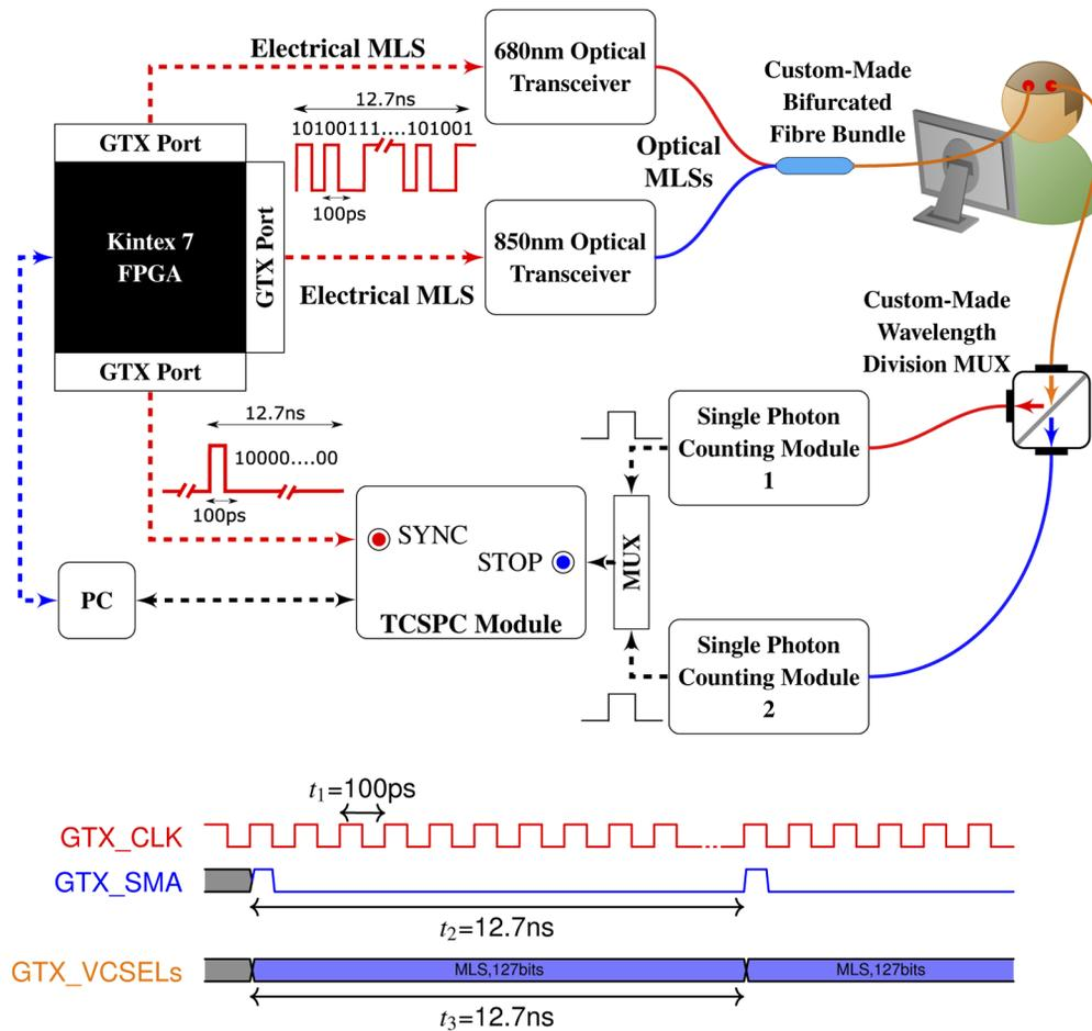
**Fig. 1.** A schematic diagram of the dual-wavelength spread spectrum-based TD system for fNIRS applications. The timing diagram at the bottom of the Figure indicates the synchronous transmission of all FPGA's GTX transmitter ports.
