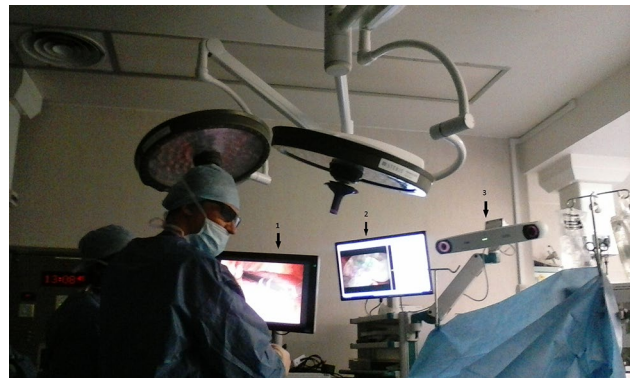
Fig. 3 The surgeon uses a standard laparoscopic screen (1) whilst the research team uses a separate screen (2) for calibration, registration and data capture. In the later phase of the study the surgeon is allowed to visualise the AR view through this screen. The optical tracking camera (3) is attached to an adjustable arm
