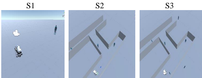
Fig. 10. Three test scenarios. S1 has one pedestrian moving towards the wheelchair, S2 has three pedestrians moving in different directions in the H maze while the number of pedestrians was increased to six in S3. All pedestrians move at an average speed of 1.1m/s
