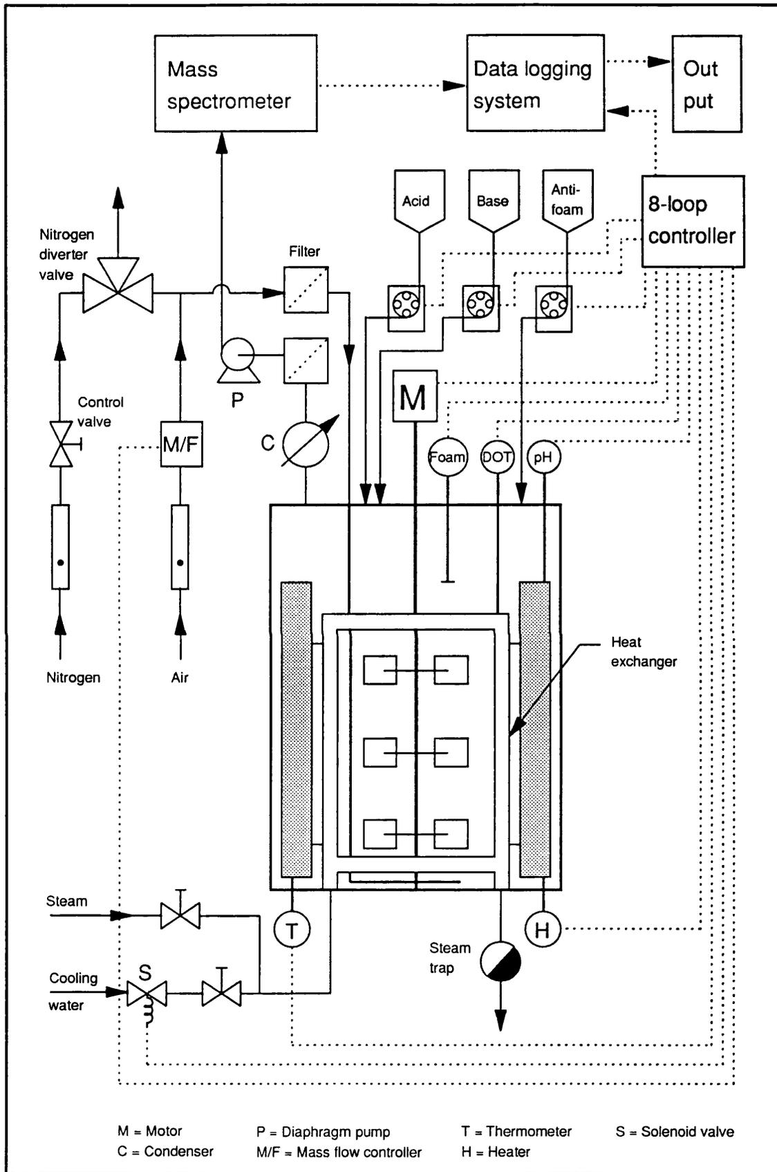
**Figure 2.1 :** Schematic diagram of 20-L LH fermenter equipped with instruments and automatic control systems.
