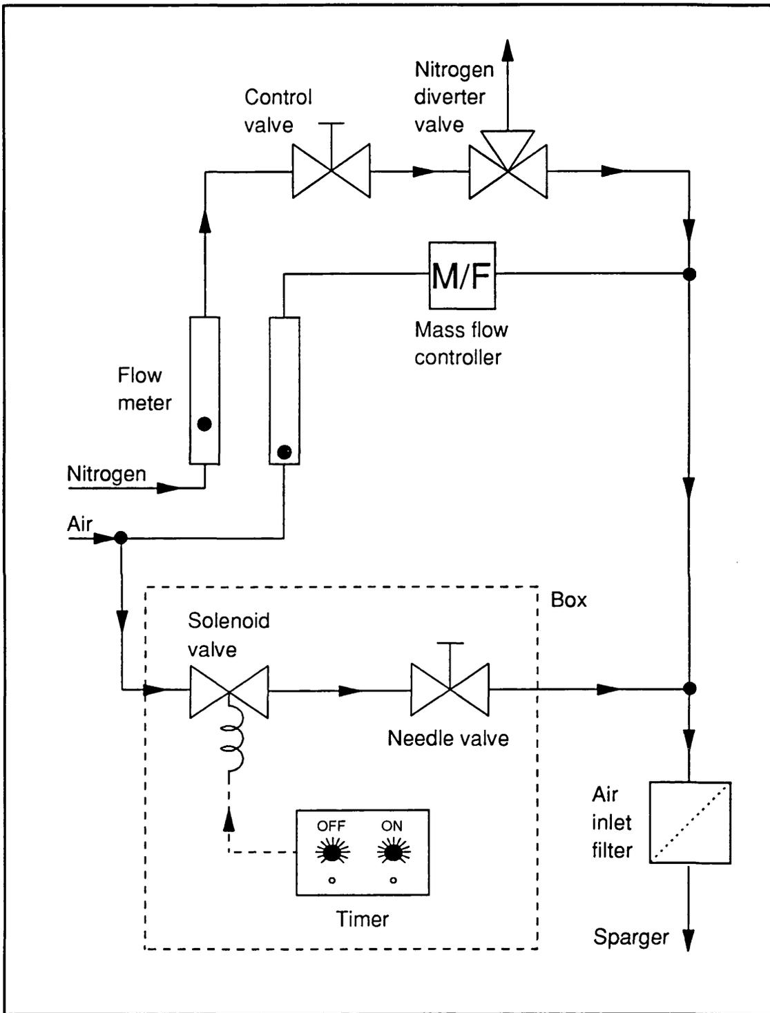
Figure 2.2 : Schematic diagram of the DOT cycling device and gas system.
