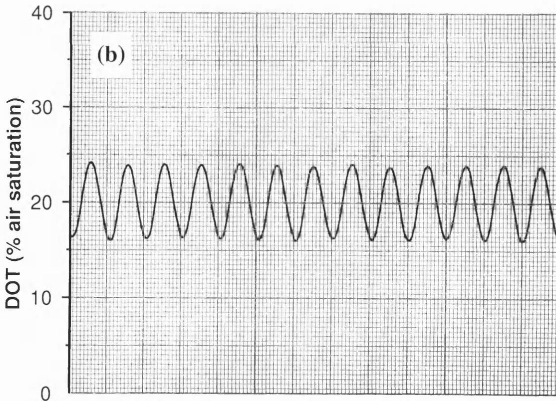
Figure 3.19 : DOT cycling traces recorded with a chart speed of 1 cm/min.
