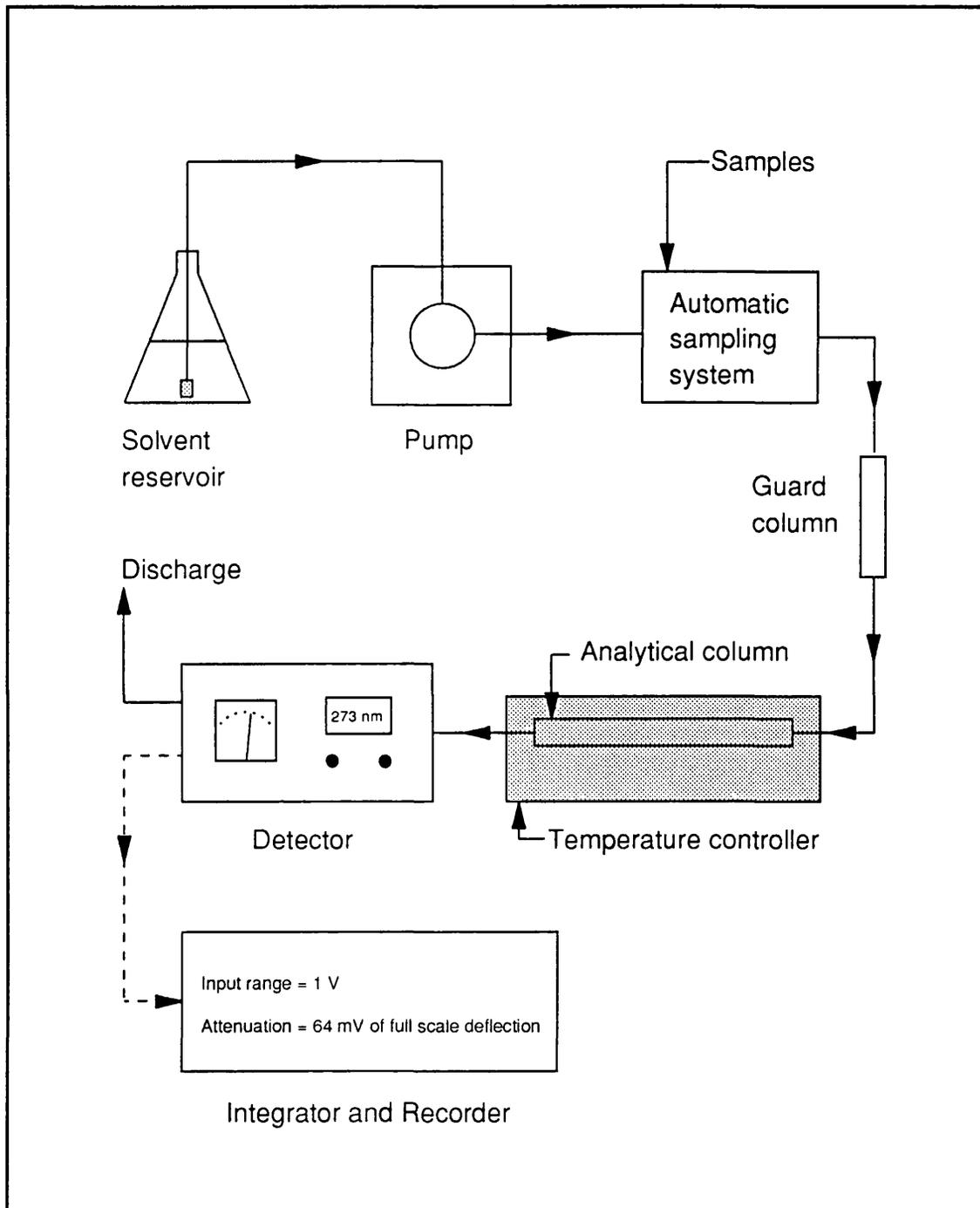
**Figure 2.3 :** Schematic diagram of the high performance liquid chromatography (HPLC).
