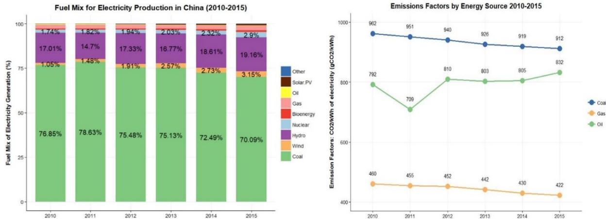
11 **FIGURE 2 China’s electricity generation mix and corresponding emission factors 2010-2015.**
