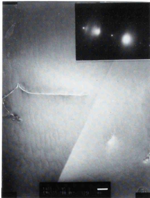
Plate 4.6 Dark field image of the same dislocation, but with g = \langle 022 \rangle . Scale bar = 200 nm.
