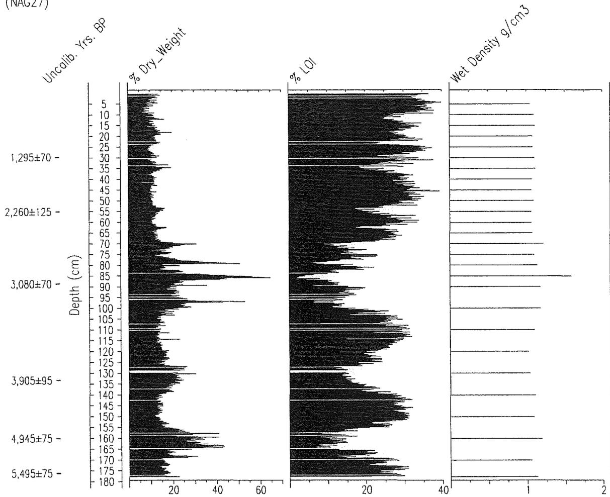
**Figure 4.1: Lochnagar (NAG27) sediment lithology, including bulk density (wet density g m<sup>3</sup>), dry matter (% dry weight) and organic matter (% LOI)**
