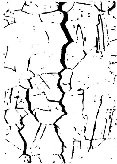
Fig. 7 : Intergranular stress-corrosion cracking of brass, taken from [19]
