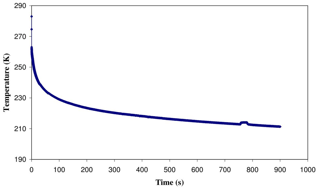
Figure 5. The discharge CO2 temperature with time following full bore pipeline rupture
