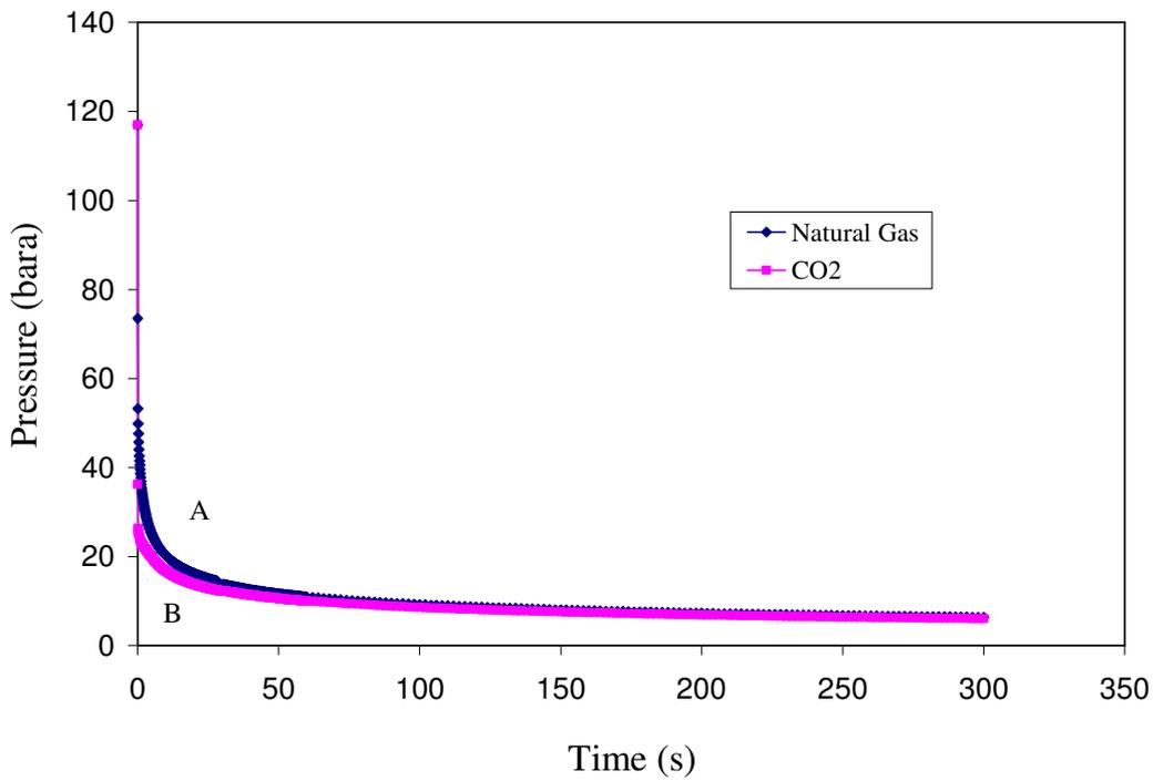
Figure 1. The variation of discharge pressure with time following full bore pipeline rupture
