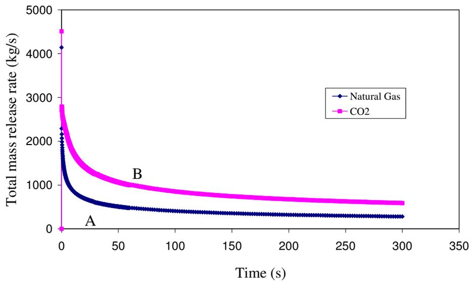
Figure 2. The variation of mass release rate with time following full bore pipeline rupture
