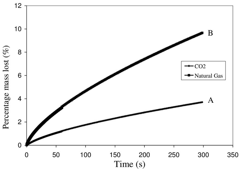
Figure 4. The variation of % mass lost with time following full bore pipeline rupture
