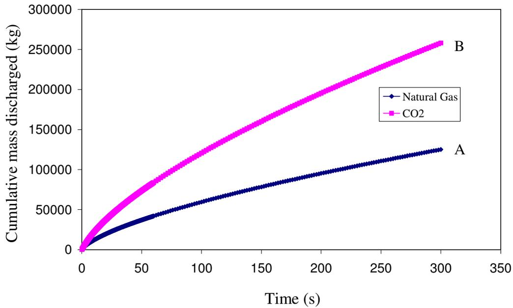
Figure 3. The variation of cumulative mass discharged with time following full bore pipeline rupture
