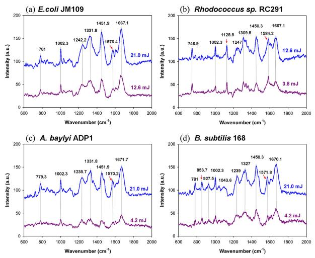
FIG 8 Raman spectra of *E. coli* JM109 (a), *Rhodococcus* sp. RC291 (b), *A. baylyi* ADP1 (c), and *B. subtilis* 168 (d) at two irradiation doses shown separately in blue and purple colors. These are averaged spectra from <10 cells. Red arrows indicate features whose positions differ significantly in the spectra of the four strains.
