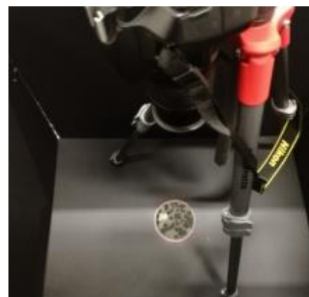
Fig. 4. Configuration created for the determination of the coverage of mould on each agar plate
