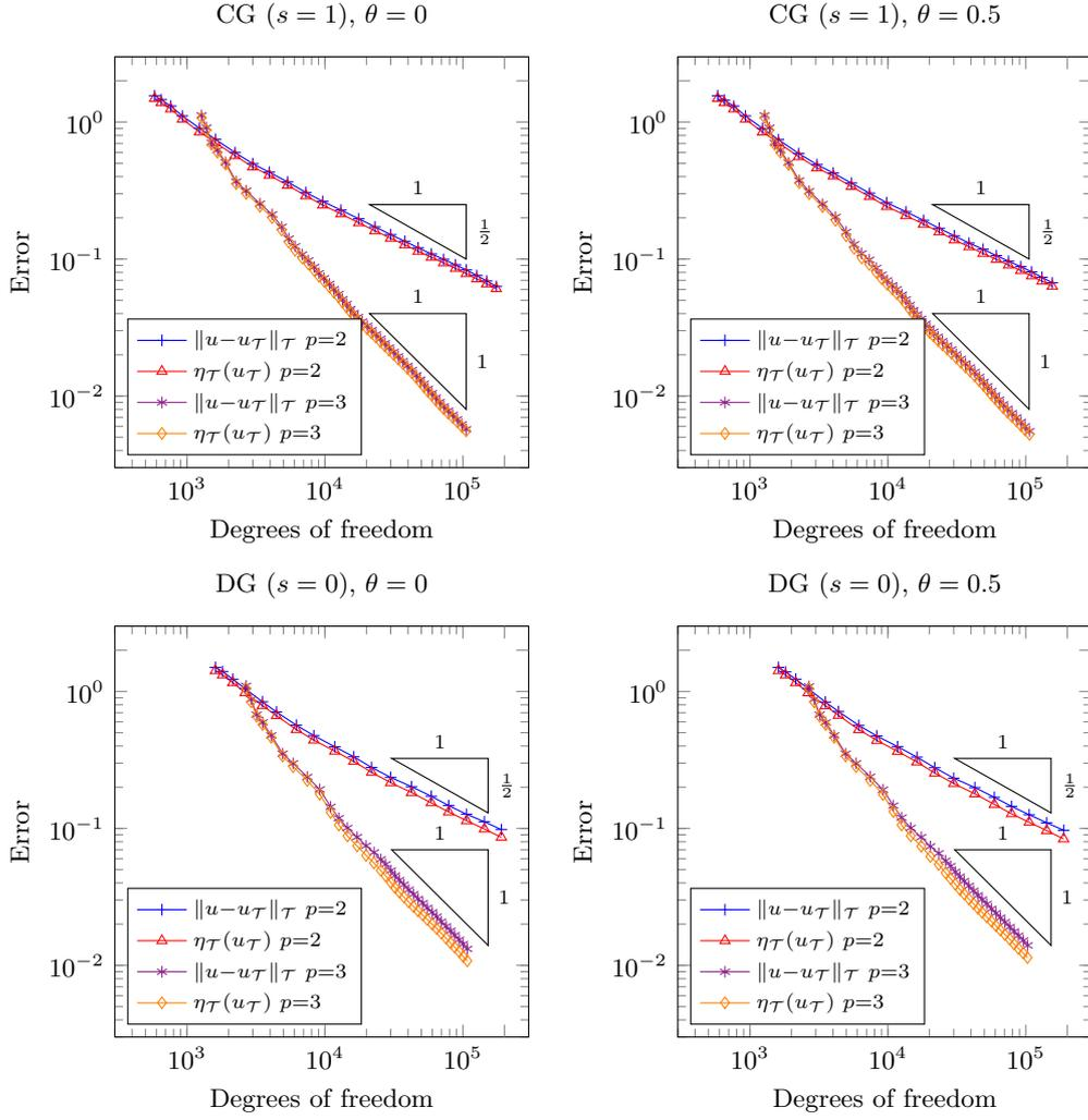
Figure 4: Experiment of Section 7: convergence plots for a range of DG and  $C^0$ -IP methods of the form of (5.9) on adaptively refined meshes. The convergence rates are optimal with respect to the number of degrees of freedom.
