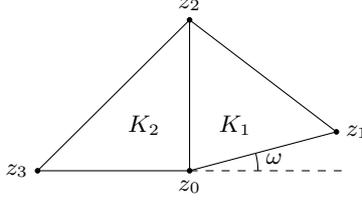
Figure 1: [Example of Remark 4.2]. A pair of elements  $K_1$  and  $K_2$  are formed by the vertices  $z_0 = 0$ ,  $z_1 = (\cos \omega, \sin \omega)$  for some  $\omega \in (0, \pi/2)$ ,  $z_2 = (0, 1)$  and  $z_3 = (-1, 0)$ . Suppose that the lower edges of  $K_1$  and  $K_2$  are on the boundary  $\partial\Omega$ , so that  $z_0$  is a corner (sharp) vertex of  $\partial\Omega$ .
