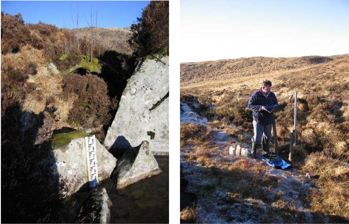
*Figure 14. a) Lake level stage board at Round Loch of Glenhead, and b) Checking the outflow level logger on 20<sup>th</sup> January and standard solutions for dilution gauging (flow calibration) (Photos Chris Curtis).*
