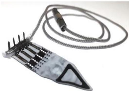
Figure 1: An example of the type of MEC used in this experiment. The example shown is a four-electrode type fitted with a Cooper cable and Lemo connector.
