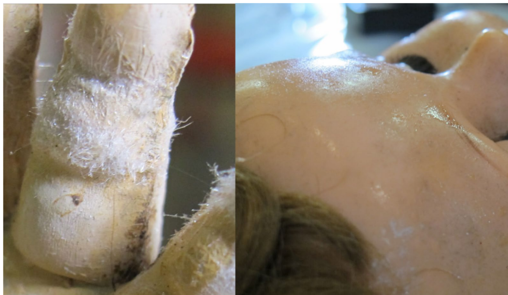
Fig. 2 (Left) Bloom of triphenyl phosphate plasticiser and (right) phthalate plasticiser exudation from dolls made of cellulose acetate. Images reproduced with permission of Tate, London. Both dolls form a part of 'Mouth Open, Teeth Showing (I)'; 2000, Zoe Leonard, Tate X717743 L04293
