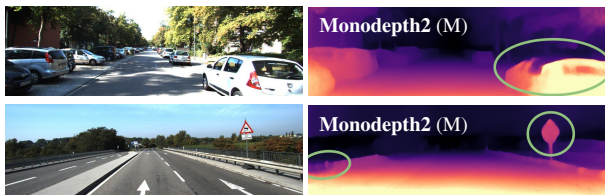
Figure 8. Failure cases. Top: Our self-supervised loss fails to learn good depths for distorted, reflective and color-saturated regions. Bottom: We can fail to accurately delineate objects where boundaries are ambiguous (left) or shapes are intricate (right).
