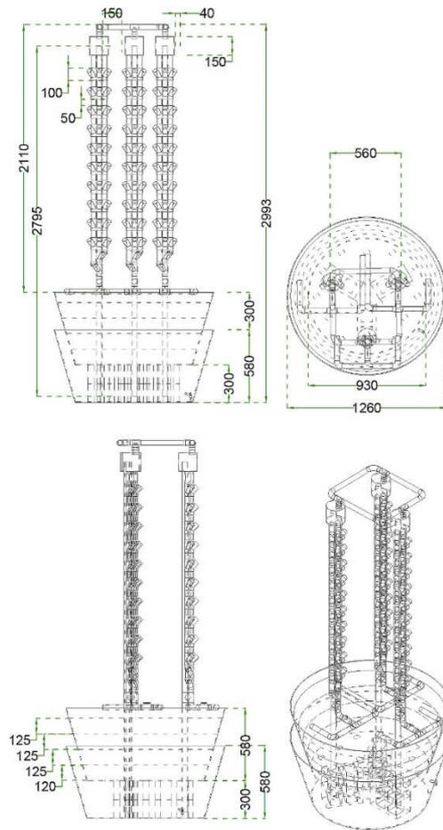
Figure S.15 - Technical drawing combined hydroponic and vermifilter unit
