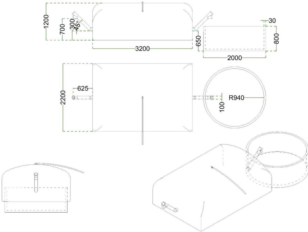
Figure S.11 - Technical drawing digester 7.5 m<sup>3</sup>
