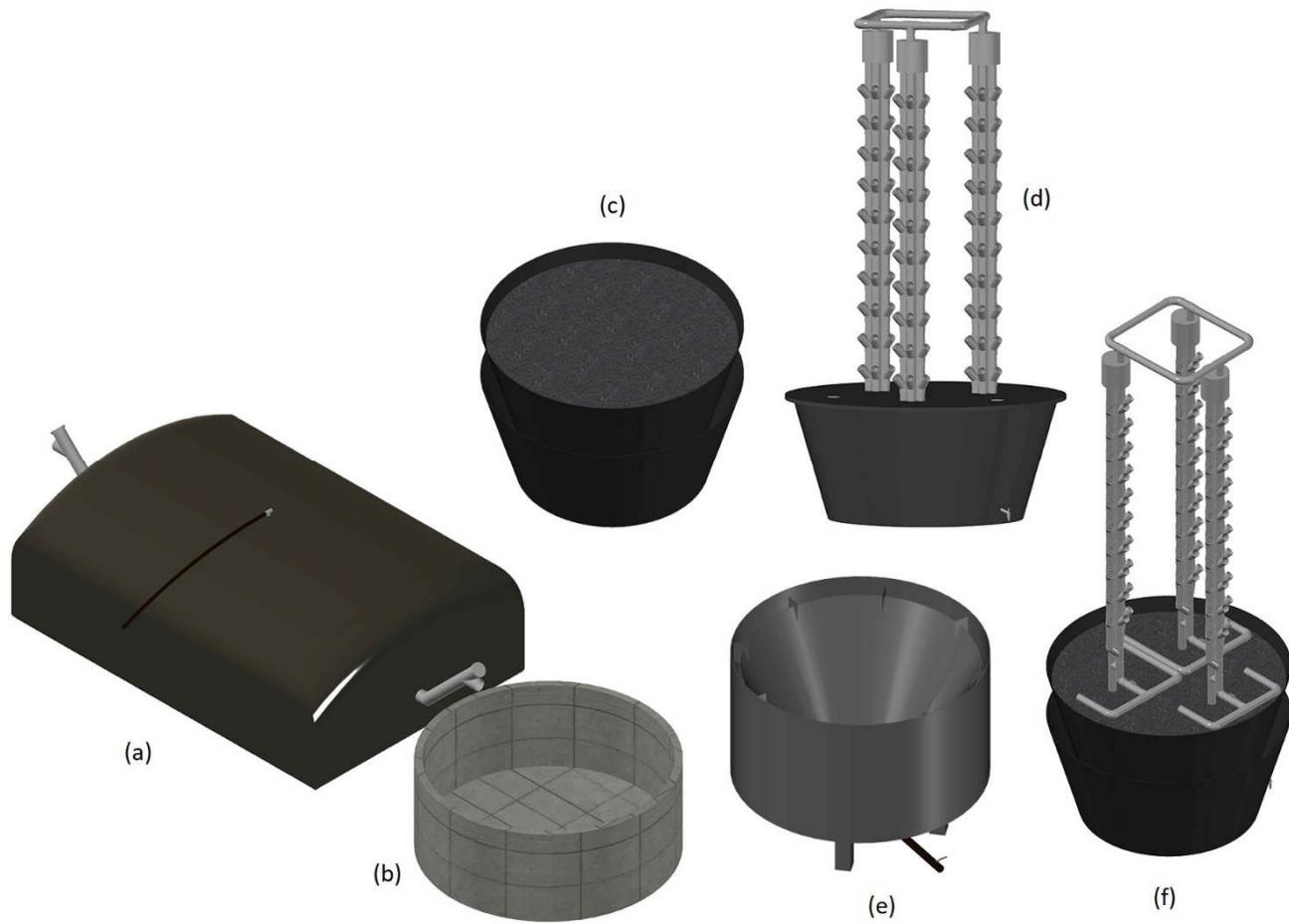
Figure 2 - Conceptual designs of the various units. (a) Anaerobic digester unit 7.5 m<sup>3</sup>, (b) Digestate storage, (c) Vermifilter unit, (d) Hydroponic unit, (e) Pyrolysis unit, (f) Combined hydroponic and vermifilter unit. The shredder is not included in this figure.
