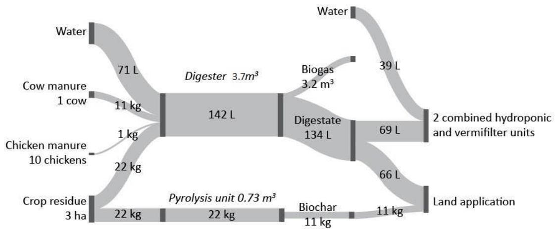
Figure 7 - Example configuration of the system with the average daily in- and outputs for a farm with 3 hectares of cropland (44 kg of crop residue per day), 10 chickens (1 kg of chicken manure per day) and 1 cow (11 kg of cow manure per day). Note that the pyrolysis unit is only used twice a month, feedstock is stored between operations.
