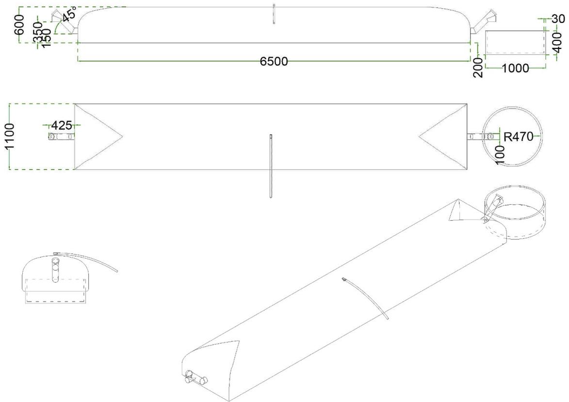
Figure S.10 - Technical drawing digester 3.7 m<sup>3</sup>
