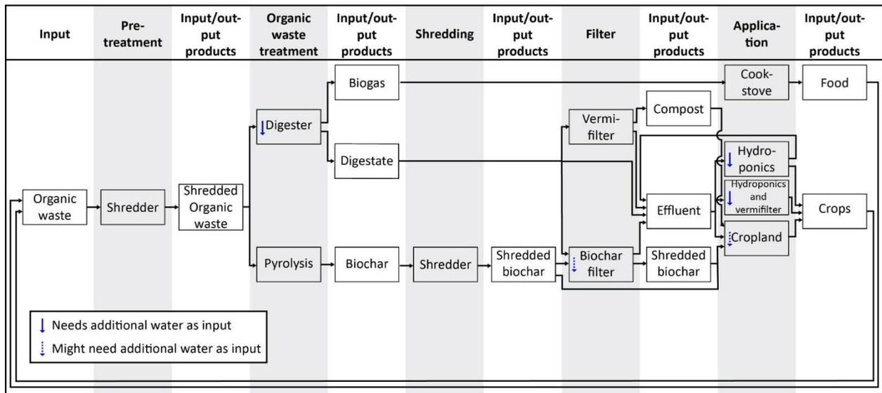
Figure 3 - Complete system design and possible configurations. Solid blue arrows indicate the need for additional water into the system.
