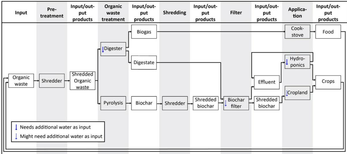
Figure 5 - System configuration with a digester 7.5 m<sup>3</sup>, pyrolysis unit and a hydroponics unit
