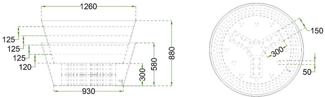
Figure S.14 - Technical drawing vermifilter unit
