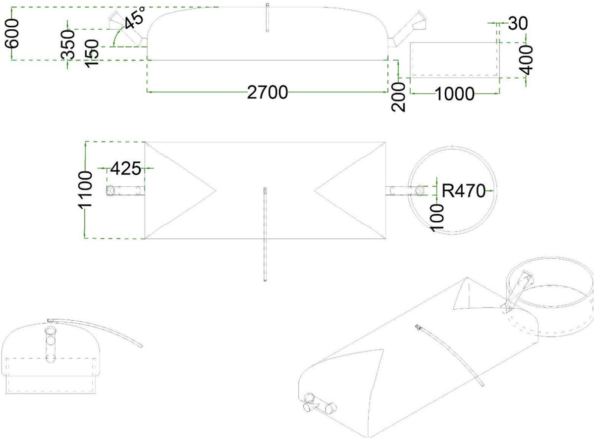
Figure S.9 - Technical drawing digester 1.5 m<sup>3</sup>
