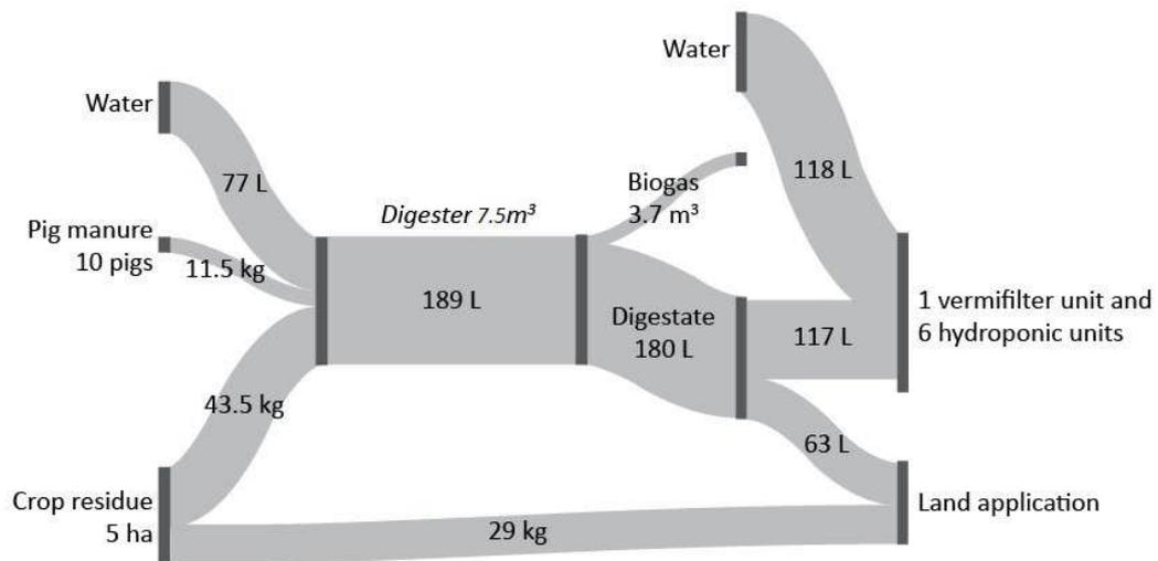
Figure 8 - Example configuration of the systems with the average daily in- and outputs for a farm with 5 hectares of cropland (72.5 kg of crop residue per day), 5 pigs (11.5 kg of pig manure per day).
