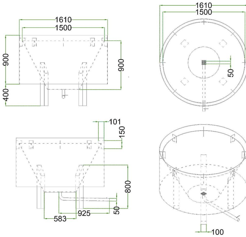
Figure S.16 - Technical drawing pyrolysis unit
