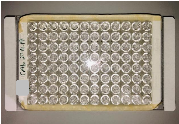
Figure 3-3: Incubation of capture antibody in 96-well microplate
