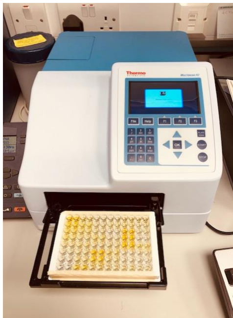
Figure 3-6: Microplate reader with study plate
