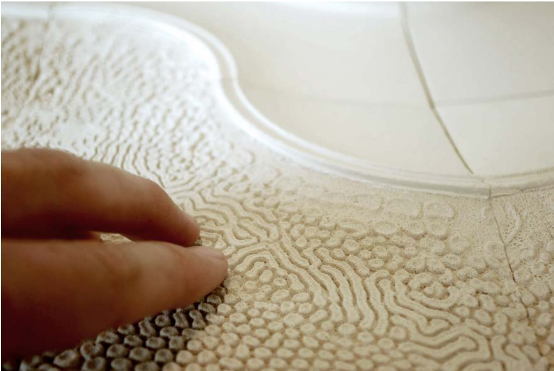
Figure 9. surface detail of probiotic tiles showing the textural, porous surface of the probiotic zone
