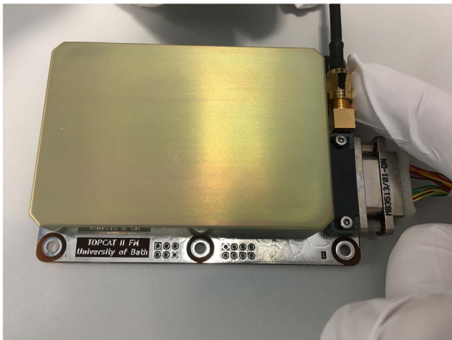
Fig. 8. TOPCAT II flight model. The shield protects the GPS receiver and electronic printed circuit board (courtesy University of Bath).
