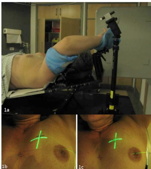
Fig. 1. a–c: The HeartSpare laser – a small laser is attached to a ball mounted grip which rotates on top of an extendable tripod. This is attached to the treatment couch using suction pads. The laser shines cross hairs on the patients' chest in free breathing (1b) and breath hold (1c). The position of the cross hairs overlying a mark placed in breath hold (as defined according to pre-treatment instructions) identifies the patient is in the correct breath hold.
