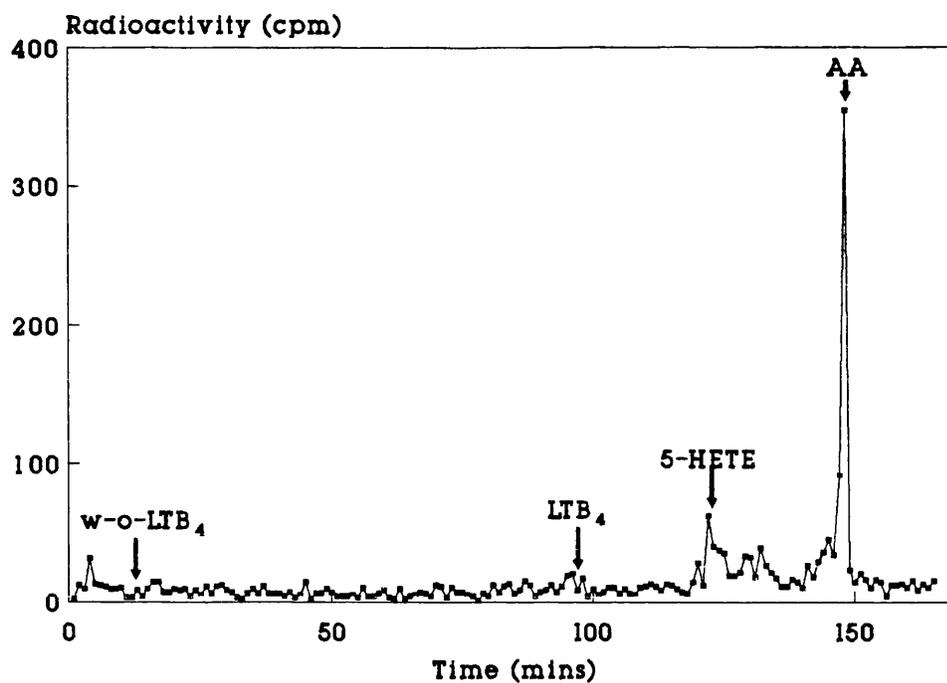
Figure 6.2b. A typical eicosanoid profile from washed neutrophils radiolabelled with  $^{14}\text{C}$ -sodium arachidonate and stimulated with  $2.5\mu\text{M}$  calcium ionophore A23187 for 4 minutes ( $n=2$ ) in the presence of  $10\mu\text{M}$  NDGA. Samples were extracted with ethyl acetate and resolved by HPLC on a gradient of 30.5-95% acetonitrile in aqueous orthophosphoric acid (pH 2.3).
