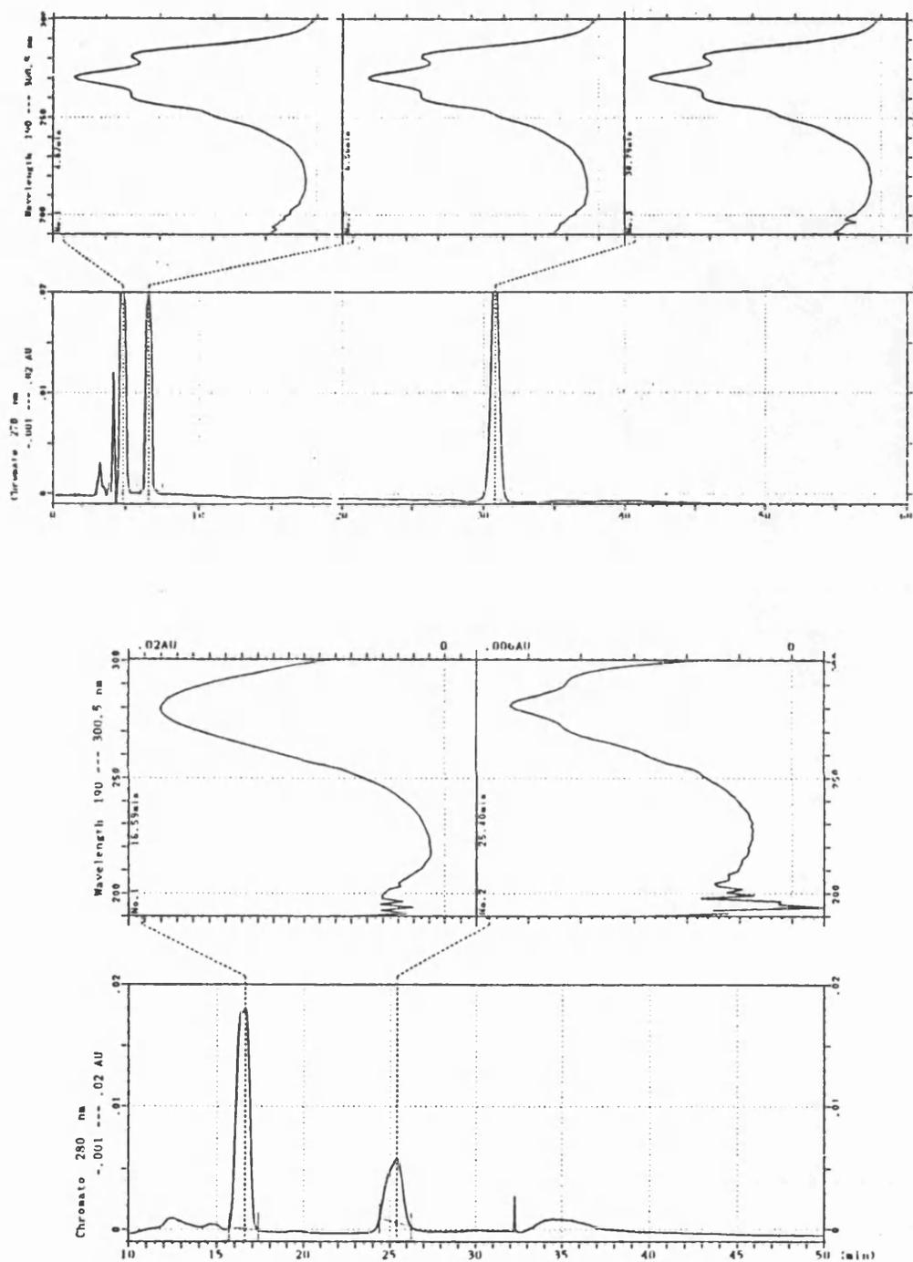
Figure 6.3. Representative absorption curves and chromatograms for standard eicosanoids. Samples (50ng of each) were chromatographed isocratically with methanol:water:acetic acid (67:33:0.1), pH 6.25, with a flow rate of 0.75ml/min. Eicosanoids identified were: from top left, OH-LTB<sub>4</sub>, COOH-LTB<sub>4</sub>, LTB<sub>4</sub>, PGB<sub>2</sub> and LTC<sub>4</sub>. Chromatograms were recorded at 270nm and peaks eluant scanned from 190-300nm.
