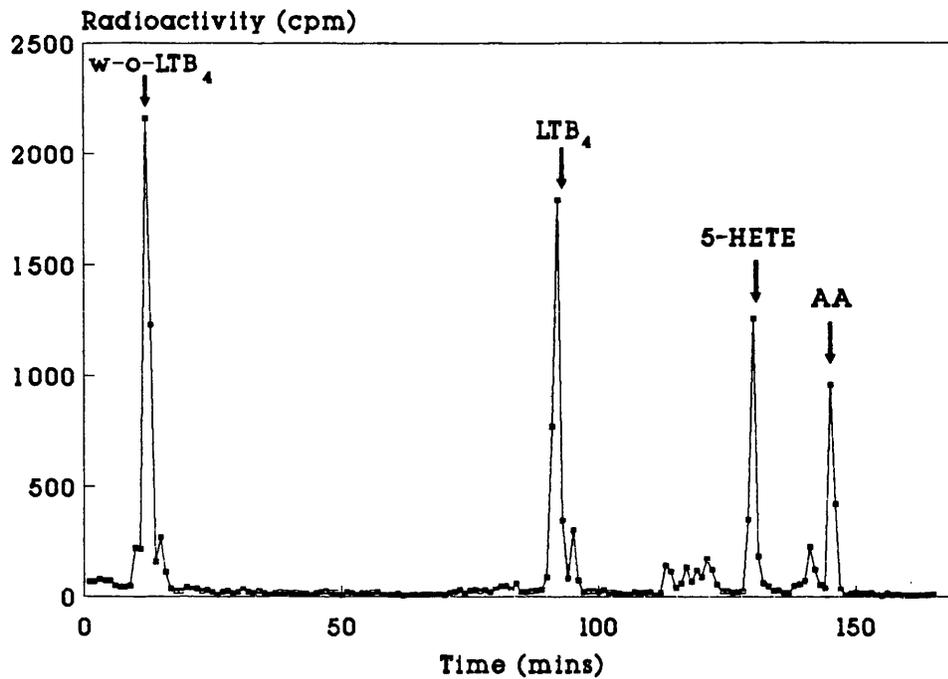
Figure 6.2d. A typical eicosanoid profile from washed neutrophils radiolabelled with  $^{14}\text{C}$ -sodium arachidonate and stimulated with  $2.5\mu\text{M}$  calcium ionophore A23187 for 4 minutes ( $n=2$ ) in the presence of  $1\text{mM}$  aspirin. Samples were extracted with ethyl acetate and resolved by HPLC on a gradient of 30.5-95% acetonitrile in aqueous orthophosphoric acid (pH 2.3).
