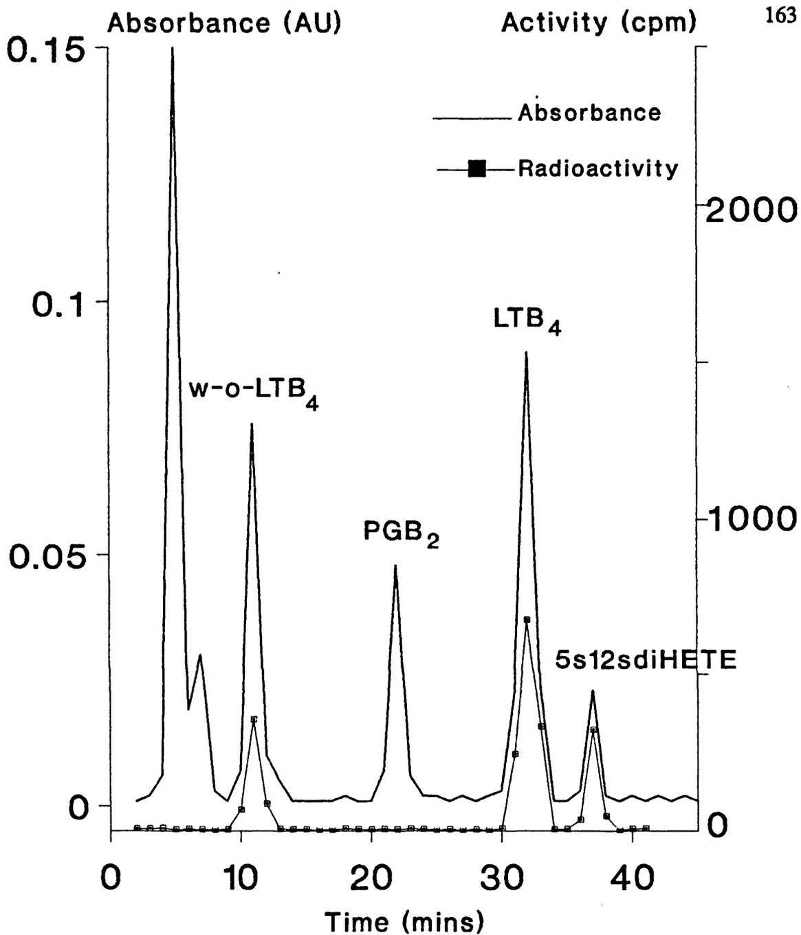
Figure 6.5c. Coincubation of <sup>14</sup>C-sodium arachidonate labelled washed platelets (800x10<sup>9</sup>/l) with unlabelled washed neutrophils (10x10<sup>9</sup>/l). Cells were stimulated with 2.5μM calcium ionophore A23187 for 4 minutes. Eicosanoids were resolved isocratically with a mobile phase of methanol:tetrahydrofuran:water:acetic acid (30:25:45:0.1), pH 5.5. The trace shown is representative of 8 separate experiments.
