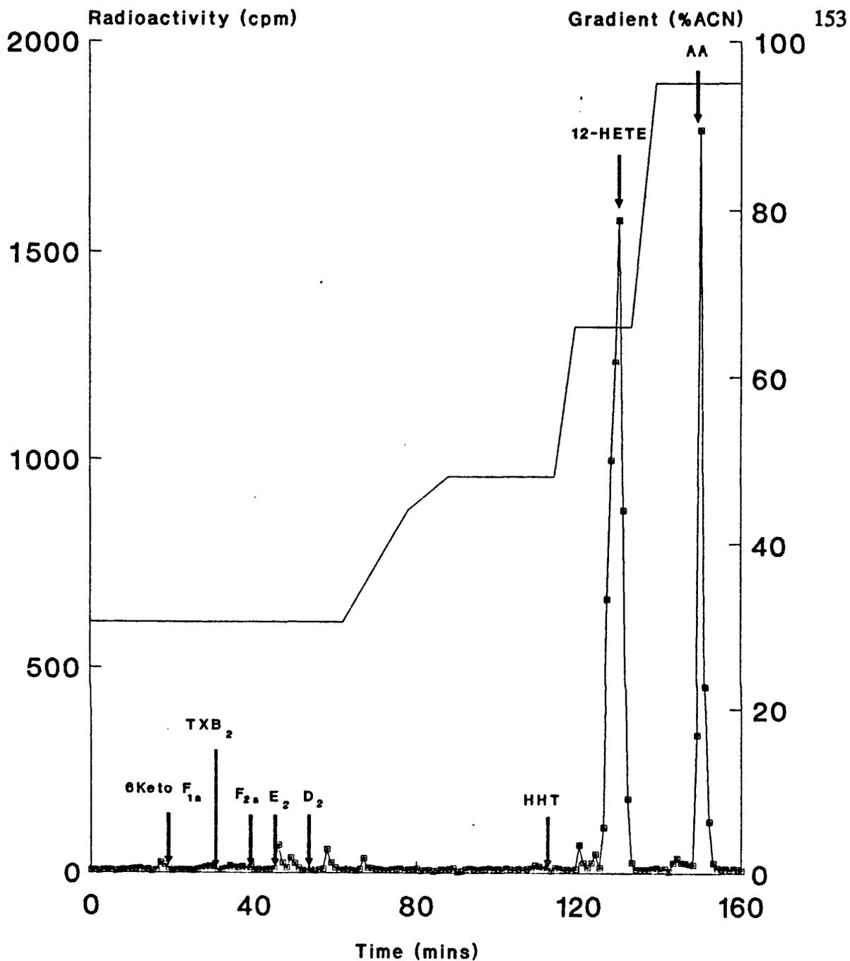
Figure 6.1b. A typical eicosanoid profile from washed platelets radiolabelled with <sup>14</sup>C-sodium arachidonate and stimulated with 20µg/ml collagen for 4 minutes in the presence of 1mM aspirin (n=10). Samples were extracted with ethyl acetate and resolved by HPLC on a gradient of 30.5-95% acetonitrile in aqueous orthophosphoric acid (pH 2.3).
