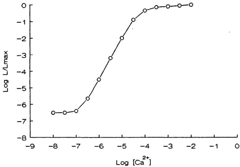
Figure 2.1 Calibration curve for determining intracellular [Ca<sup>2+</sup>] in washed, purified platelets using aequorin luminescence signals.
