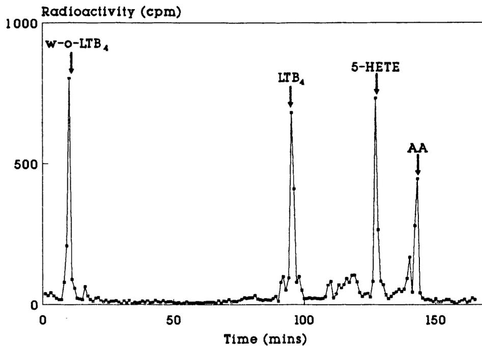
Figure 6.2a. A typical eicosanoid profile from washed neutrophils radiolabelled with <sup>14</sup>C-sodium arachidonate and stimulated with 2.5 μM calcium ionophore A23187 for 4 minutes (n=8). Samples were extracted with ethyl acetate and resolved by HPLC on a gradient of 30.5-95% acetonitrile in aqueous orthophosphoric acid (pH 2.3).
