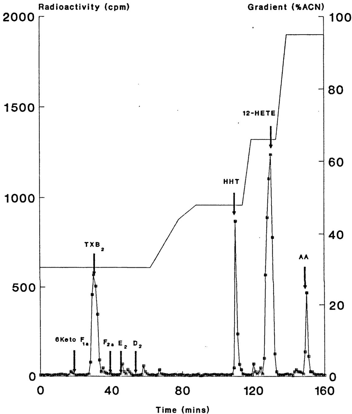
Figure 6.1a. A typical eicosanoid profile from washed platelets radiolabelled with  $^{14}\text{C}$ -sodium arachidonate and stimulated with  $20\mu\text{g/ml}$  collagen for 4 minutes ( $n=10$ ). Samples were extracted with ethyl acetate and resolved by HPLC on a gradient of 30.5-95% acetonitrile in aqueous orthophosphoric acid (pH 2.3).
